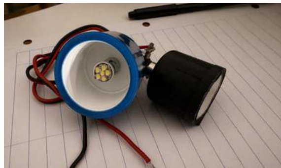
Photo 2: Modern LED lighting fixture
